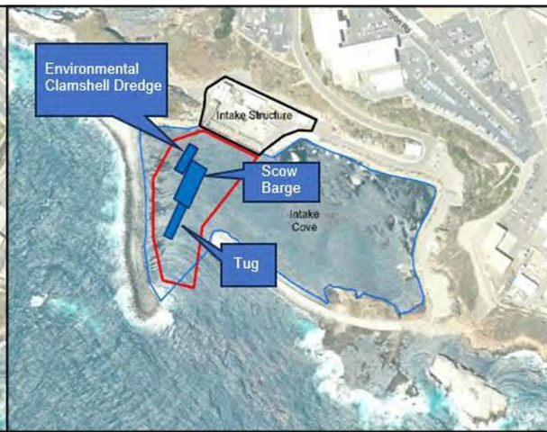
Figure 1b: Possible locations of clamshell dredge equipment.
